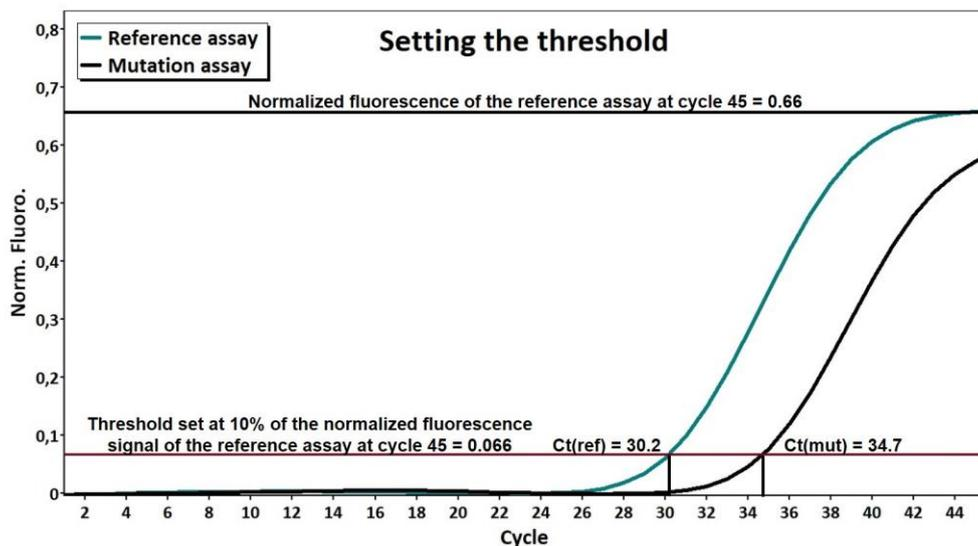
**Figure 2:** Setting the threshold. Read the fluorescence value for the reference assay at cycle 45 and set the threshold at 10% of this value. This setting for the threshold is now used for the analysis of the corresponding mutation assay. In the shown example,  $Ct(\text{reference})=30.2$  and  $Ct(\text{mutation})=34.7$ . Thus, the sample is positive for the mutation analyzed.
