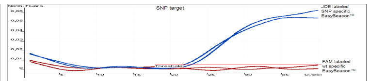
SNP detection with HydroEasy™ probes. Duo-plex reaction with probes for both the wild type and the Single Nucleotide Polymorphism
